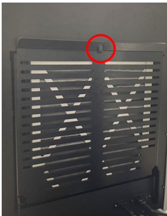
Figure 18. Air filter cover with the release tab circled in red.
