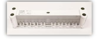
c. Tilt combined apparatus slowly 90° clockwise while it continues to rest on the surface. The tubes will now be horizontal and visible to the user.
