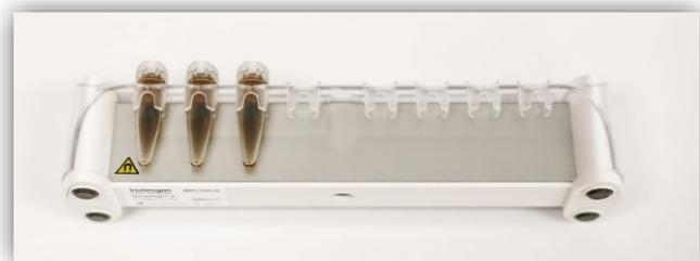
d. Tilt combined apparatus slowly 90° clockwise while it continues to rest on the surface, so that it stands fully upright, and tubes are facing the user.
