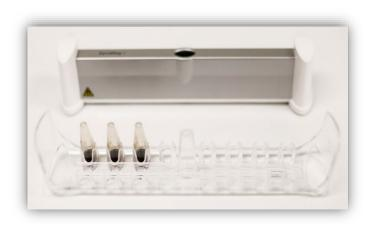
b. Invert Dynamag magnetic base and lower onto clear rack.
