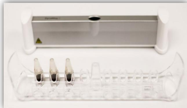
b. Invert Dynamag magnetic base and lower onto clear rack.
