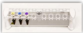
e. Make sure the Nanobind Disk is held to the magnet near the top of the liquid level.
