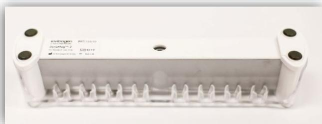
c. Tilt combined apparatus slowly 90° clockwise while it continues to rest on the surface. The tubes will now be horizontal and visible to the user.
