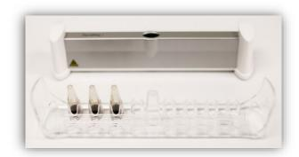
b. Invert Dynamag magnetic base and lower onto clear rack.
