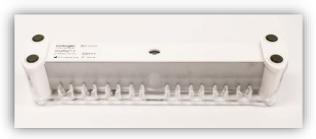
c. Tilt combined apparatus slowly 90° clockwise while it continues to rest on the surface. The tubes will now be horizontal and visible to the user.
