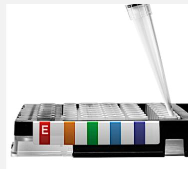
7. Typically the full 200 µL of sample cannot be recovered. 75–125 µL is the expected range.
