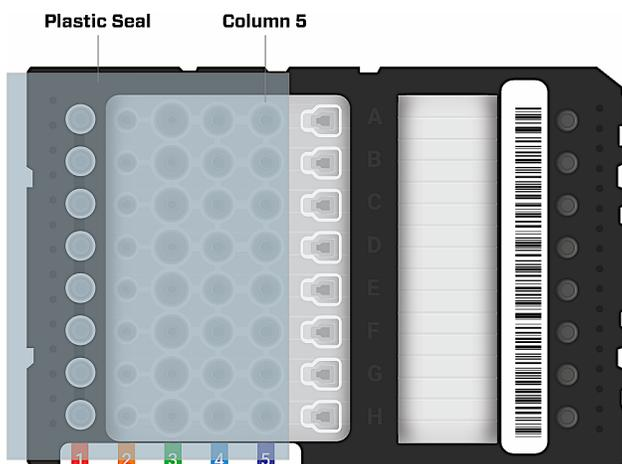
3. Cover Columns 1–5 with the plate seal while paying particular attention to ensuring a tight seal for each well in Column 5.
