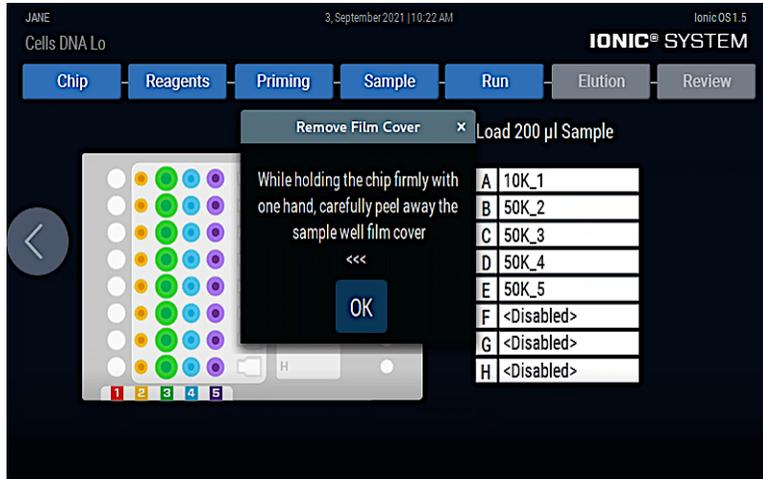
5. While gripping the chip appropriately on the side skirt, hold the chip securely against the chip holder and carefully peel off the adhesive cover over the sample wells using the pull tab.
