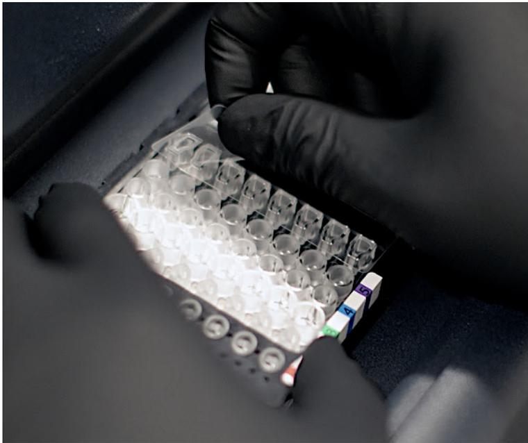
6. Using a P200 pipette, dispense **200 µL of sample** to each sample well with the tip inserted **no more than 50%** into the well. Slowly retract pipette tip from the well while dispensing to keep tip positioned at the surface of the fluid filling into the well.
