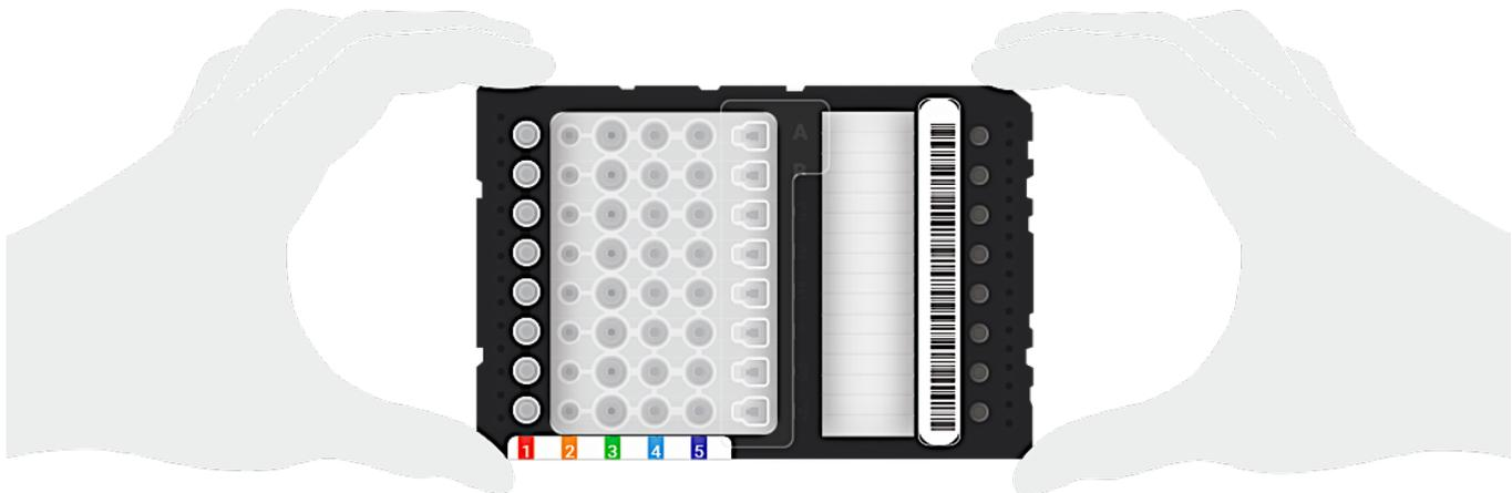
3. Identify the notched corner of the chip and orient the chip such that the notch is at the upper right-hand corner (see **FIGURE 6**).
