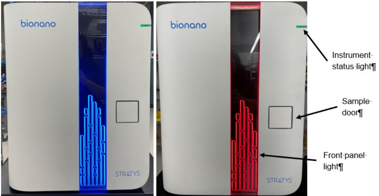
Figure 2. When the front panel light is illuminated red (right panel of figure), the instrument is not safe to run. Turn the instrument off and contact Bionano Support.
