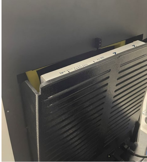
Figure 18. Air filter cover opened with air filter exposed.
