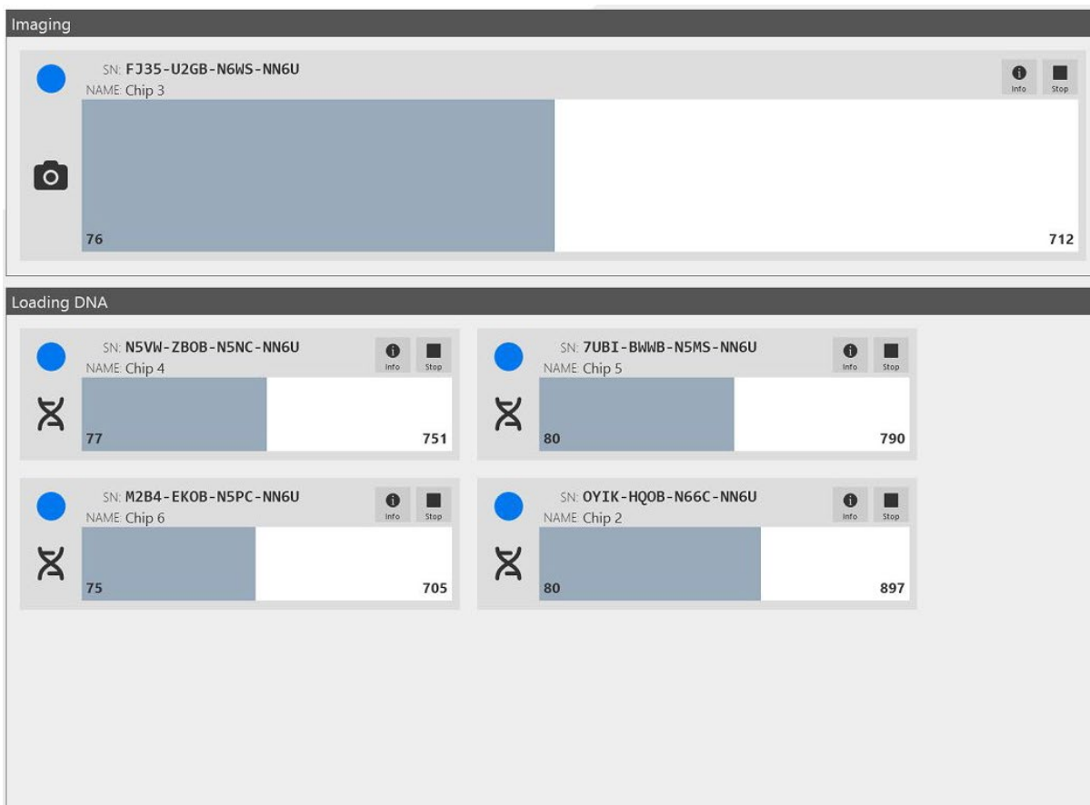
Figure 12. During the run, the software shows the state of each chip as well as the progress towards completing data collection. The blue dot next to the chip indicates the Stratys Core Chip. The mint dot next to the chip represents the Stratys Plus Chip. A yellow border around the blue or mint circle indicates a priority run.
