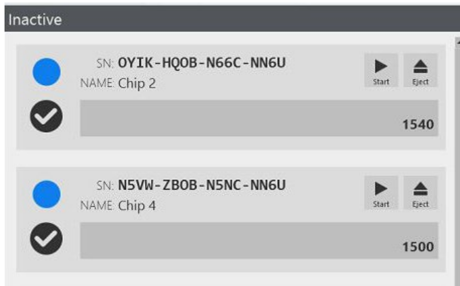
Figure 14. To eject the chip, press the Eject button next to the corresponding chip.
