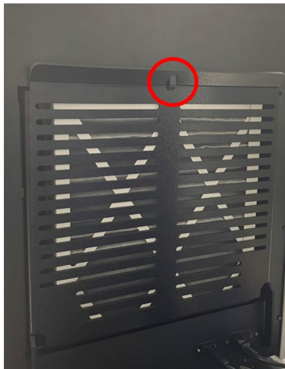
Figure 17. Air filter cover with the release tab circled in red.
