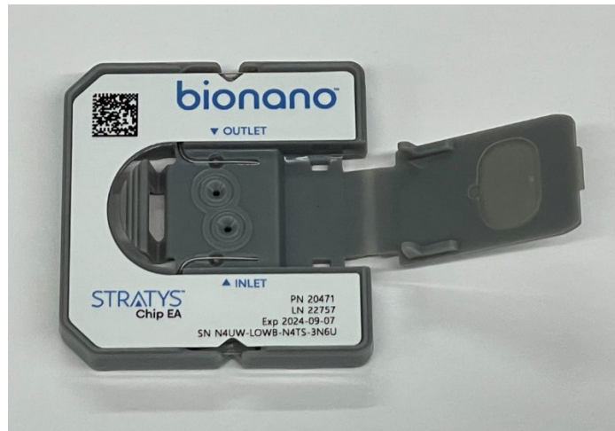
Figure 4. Stratys™ Chip with opened lid, showing the inlet and outlet ports.
