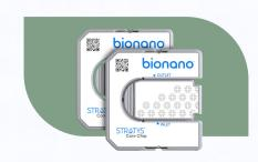
Stratys chips provide a nanofluidic environment in which DNA molecules linearize across hundreds of thousands of nanochannels where they can be imaged to reveal the underlying genomic structure and structural variation.
