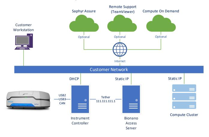
The Instrument Controller has been designed to limit and reduce the attack surface by disabling unnecessary operating system services and disabling all unsolicited incoming network traffic. Saphyr can be configured to run in kiosk mode which blocks user access to the operating system and only allows interaction with the Instrument Control software. This is the recommended operating mode in high security settings.
