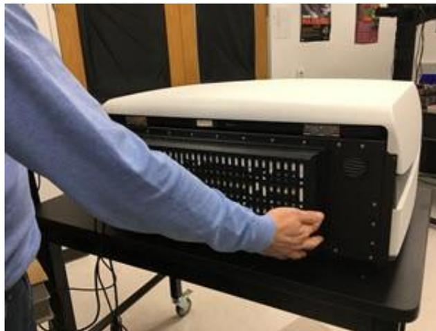
3. Remove the air filter from its cover.
