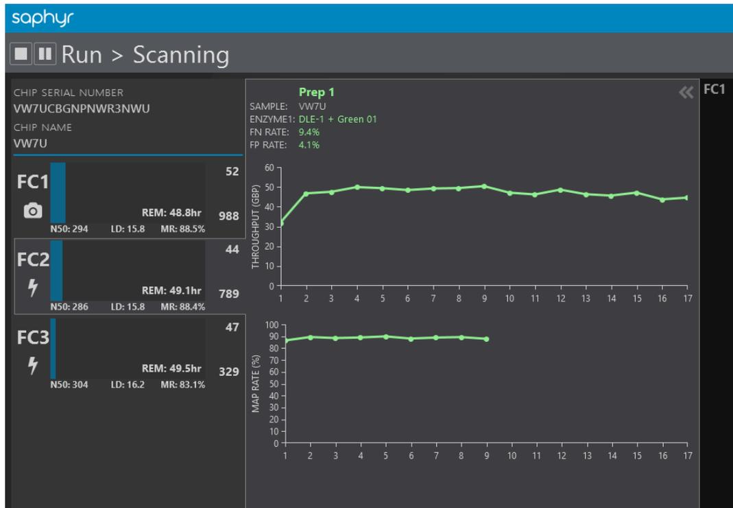
When the chip run is complete, if there is another chip (“pending”) in the instrument, it will automatically start running. The pending chip will be shown on the bottom left of the screen.
