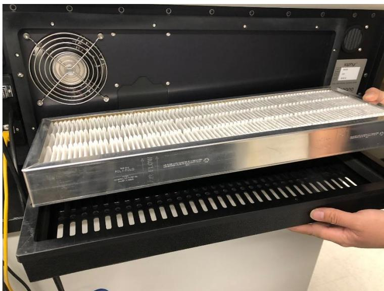
5. Attach the cover with the new air filter to the instrument.
